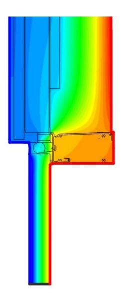
In general \_\_\_\_\_ is a 2D steady state thermal bridge analysis software using FEM (triangle elements) with an optimized conjugate gradient solver and adaptive remeshing.
