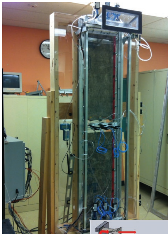
FIGURE 2: AIR FLOW EXPERIMENTS CONDUCTED TO CHARACTERIZE AIR PERMEABILITY OF DRAINAGE COMPONENTS.
