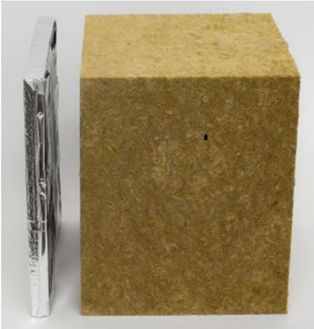
Mineral Wool is 8 to 10x thicker to deliver an equivalent R-value to VIP
