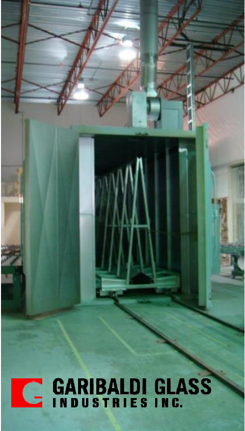
Heat Soaking can identify NiS inclusions
