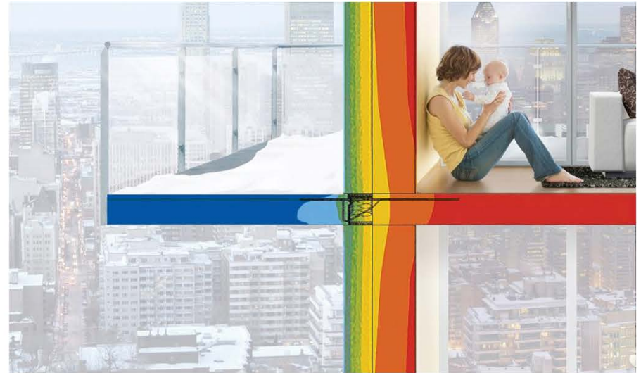
Thermally Broken Balcony
