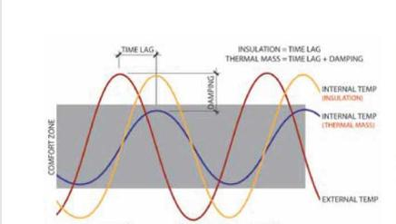
**Figure 3. Time lag and thermal damping.**
