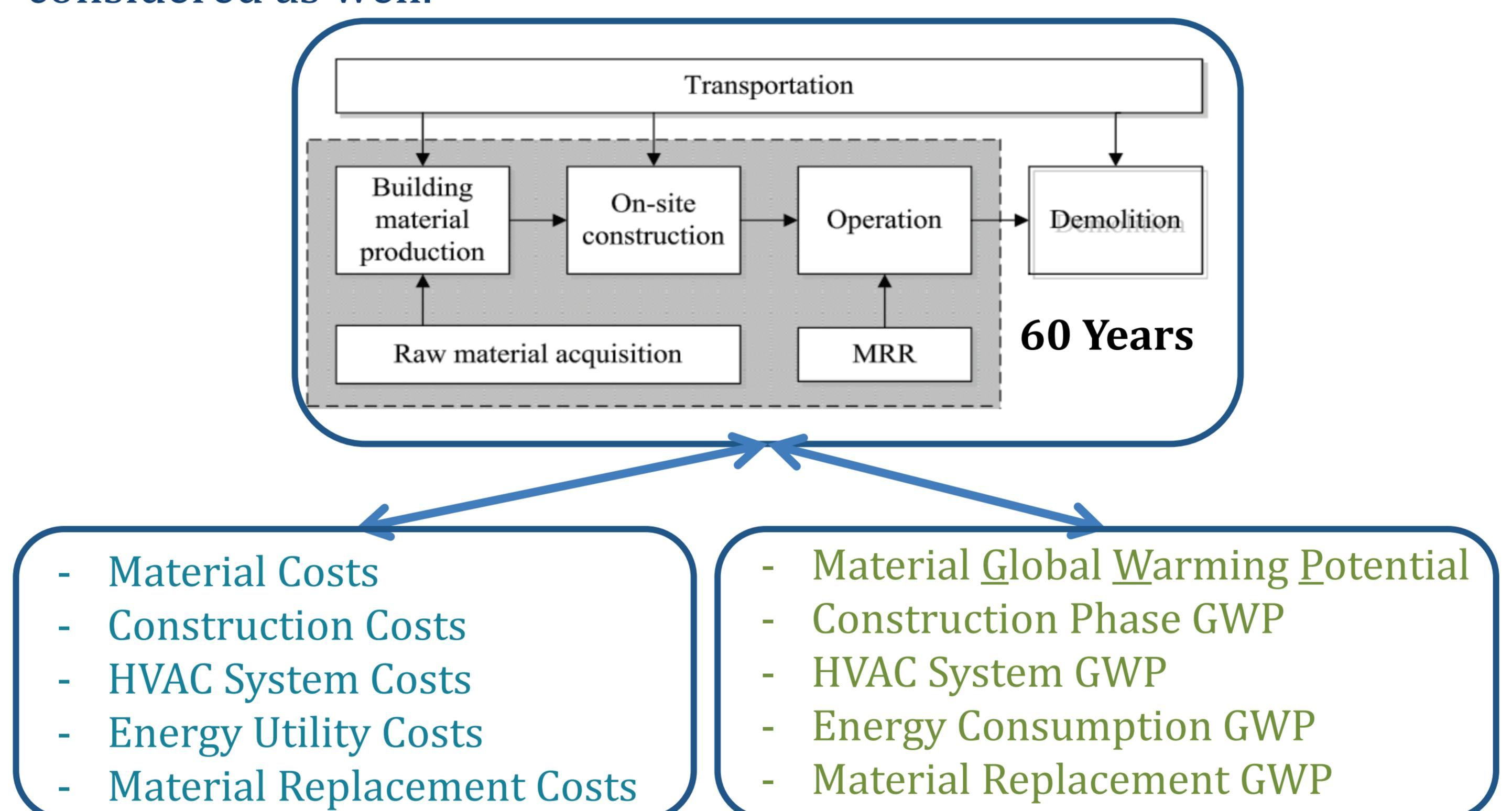
When the entire building life cycle is considered during early phase design, significant cost and environmental impact can be reduced, while ensuring energy efficiency and overall build quality.
