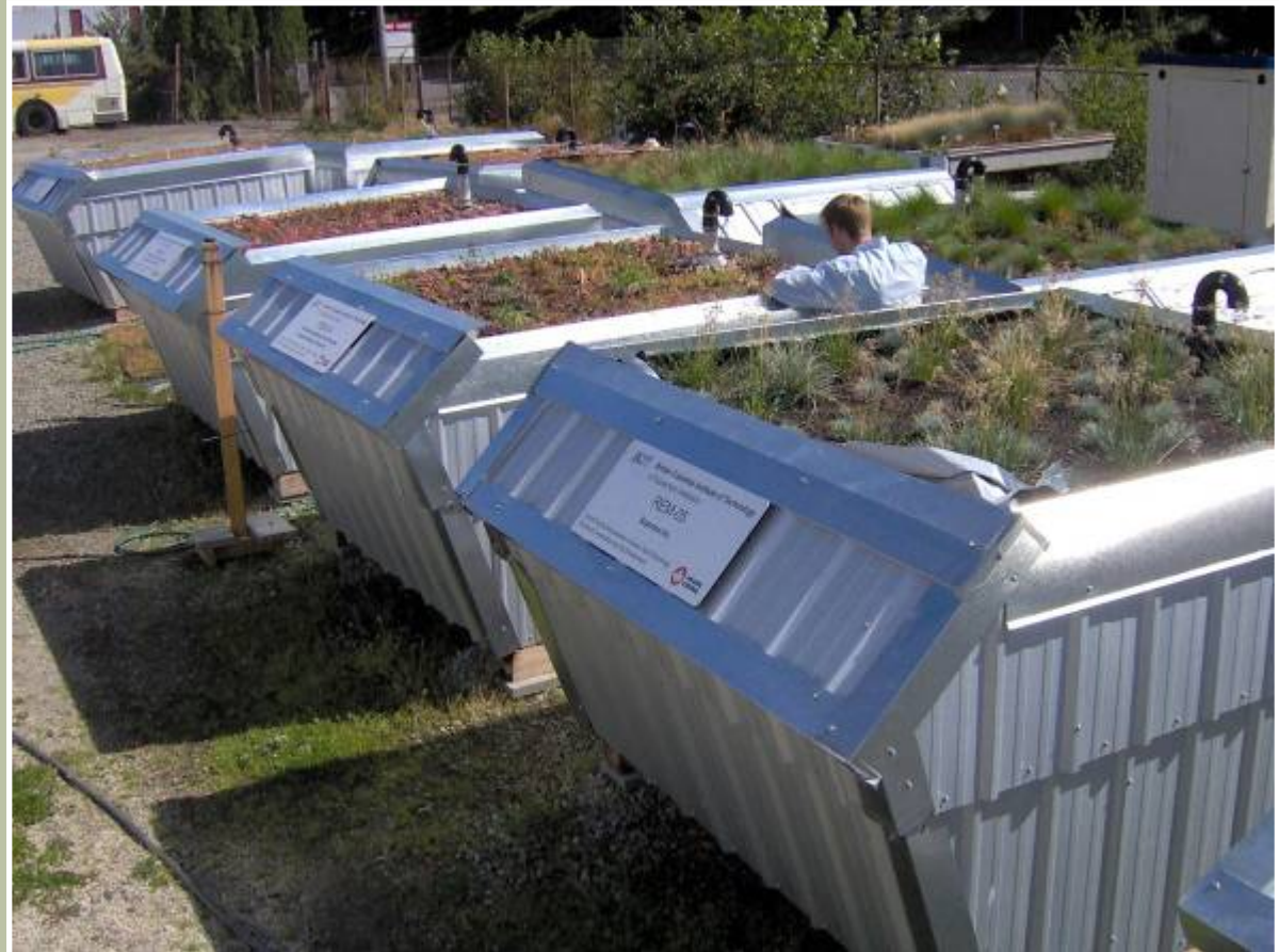
Roof Evaluation Modules at BCIT
