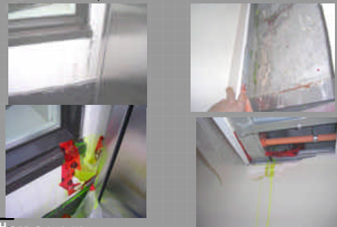
Case Study 3 – Dye test of unsealed crack between up stand curb and wall
