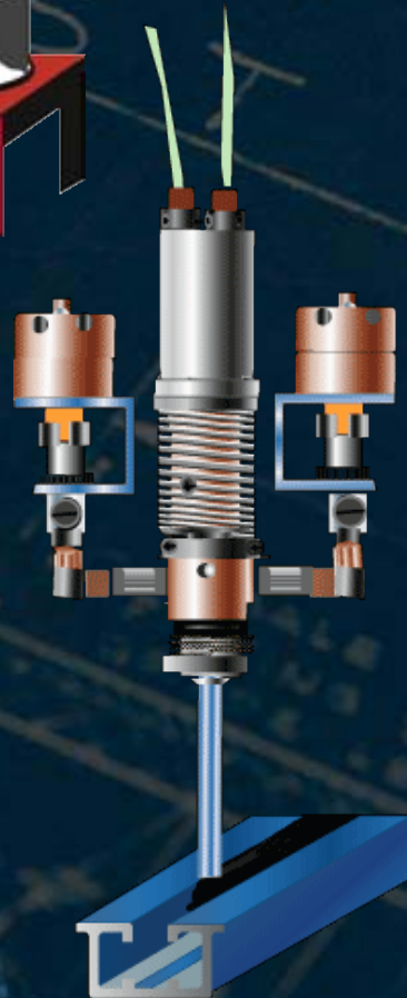
Poured and debridged thermal barrier
