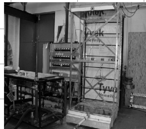
Figure 3. Airflow manifolds connected to test panel on counterbalance system (Burnett et al [2004])
