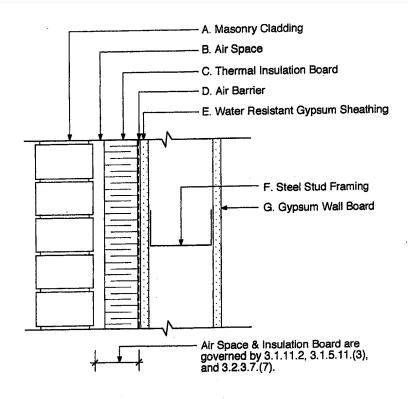
Generic Rain Screen Wall Assembly C, D, E, G have combustible components as permitted by 3.1.5.2 to 3.1.5.19.
