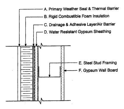
Proprietary Exterior Wall System Conforming to CAN/ULC-S134 A, B, C, D, F have combustible components.
