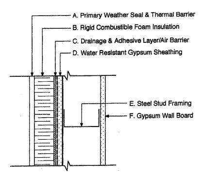
Proprietary Exterior Wall System Conforming to CAN/ULC-S134 A, B, C, D, F have combustible components.
