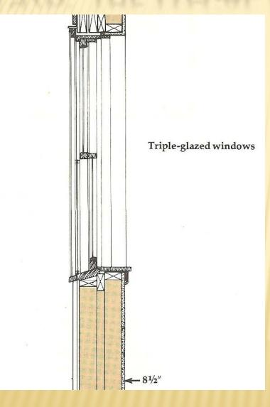
× Long axis of the house is oriented east-west. × Double 2x4 walls (R-30) × R-33 ceiling × Triple-glazed windows × An air-to-air heat exchanger
