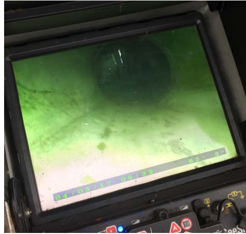
Photos 14 & 15: Example of camera'ing of a drainage system: relatively clean pipes.
